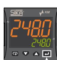
Press **■** for 3 seconds to access the configuration mode
