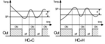
In the event of probe error, it is possible to set the instrument so that that the output "Out" continues to work in cycles according to the times programmed in the parameter "t1" (activation time) and "t2" (deactivation time).
