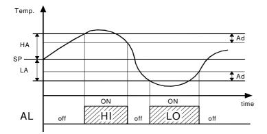
The maximum and minimum temperature alarms can be disabled by setting the relative parameters "HA" and "LA" = oF.
