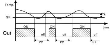
Third control (par. "P3") foresees an inhibition to the activation of the output "Out" by a time delay that starts when the output was turning on last time (delay between switching-on).
