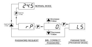
**Note:** If the Password gets lost, just cut off the supply, push P key and keeping it pressed for 5 seconds whilst switching on the supply to the instrument.
