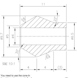
You need to use the cone In the picture above on a hole of about Ø6 - Ø7 with sharp edge, place on the same axis of the transducers hole, i.e. of the fillet
