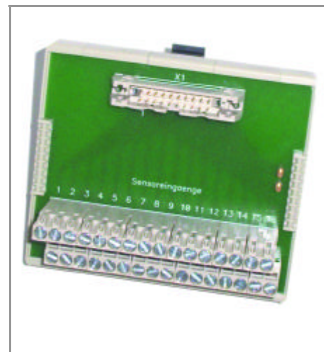
Interchange module for 16 channels with 32 screwclamps (sensor inputs) Output: 20 pole plug connector (picture similar)
